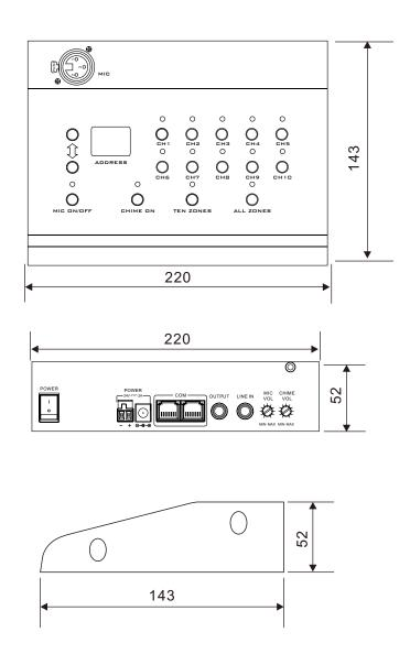
Keep the unit's all sides over 10 cm away from objects that may obstruct air flow to prevent the unit's internal temperature rise.
